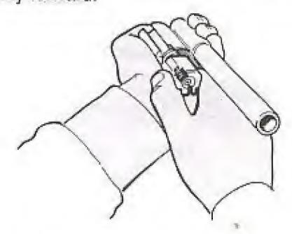
Grasping the carrier and bolt assembly firmly, turn the bolt clockwise until the slotted relief on the bolt is at the bottom position. Once again squeeze the bolt rollers to be sure they are in the fully depressed position. The bolt carrier and bolt assembly may now be inserted into the receiver.
